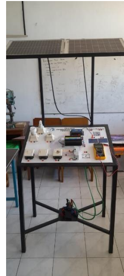
Gambar 2. Trainer Solar Panel
